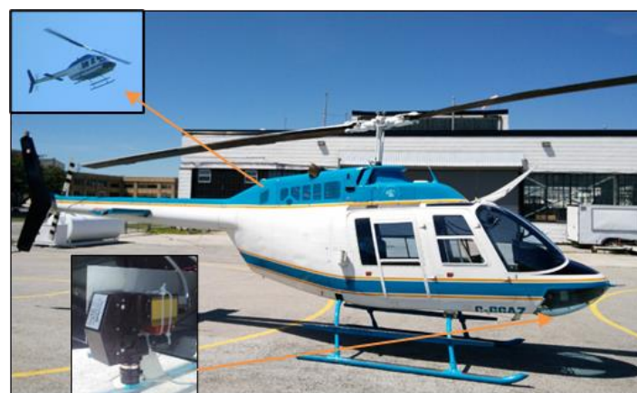
Figure 3. Helicopter and hyperspectral sensor used for imaging.
